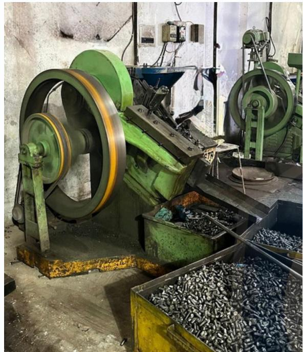
For cold forged bolts we have different threading machines as per their size requirements. These machines can feed bolts for threading automatically or manually.
