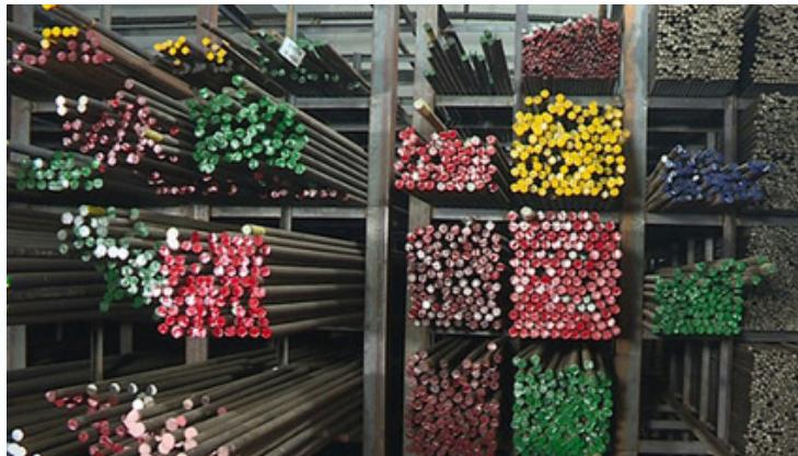
Raw material of different grades placed in different section with colour coding & quality marks
