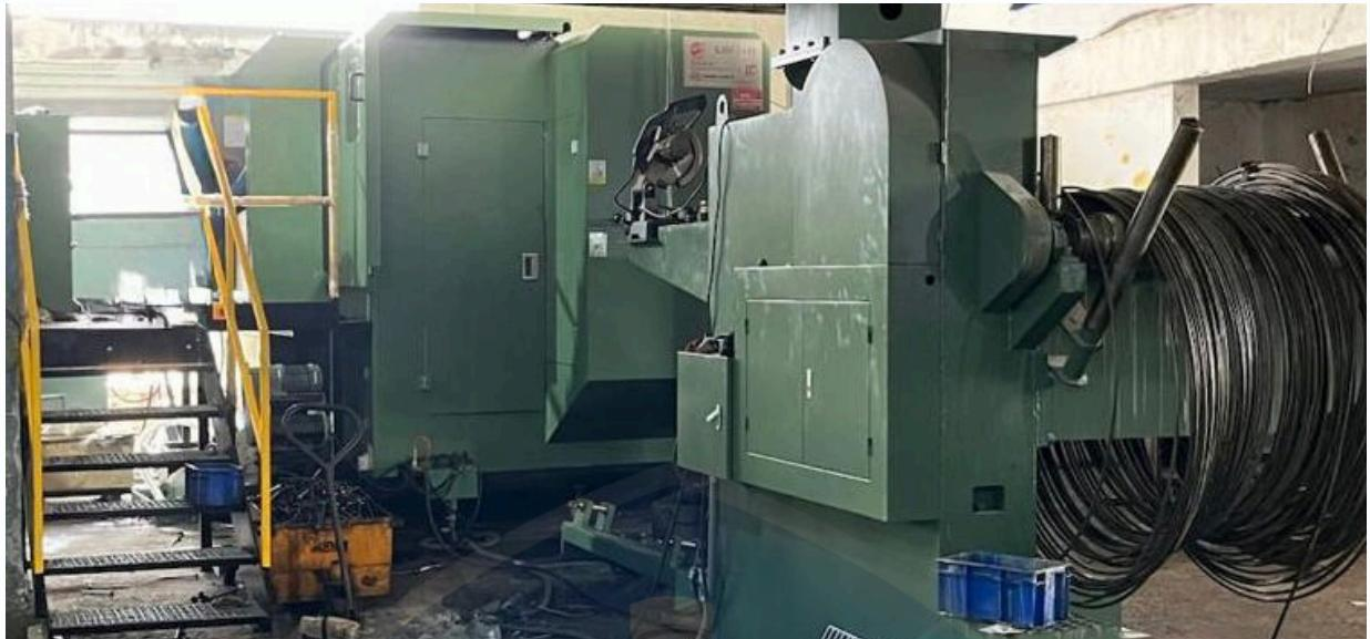
In this section, we have capacity to make bolts from M6 to M20 by cold forging. With various requirement of Bolts with different heads, we have option to make them either on Bolt forming machine or Header machine.
