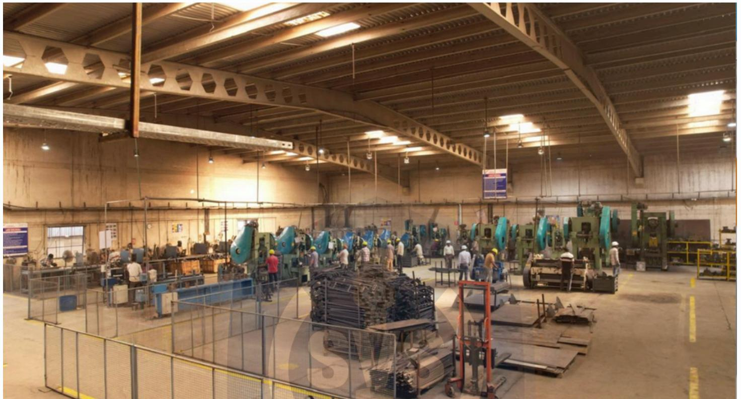
We have more than 25 hydraulic & power press machines. The maximum capacity of our press machine is 200 MT. These press machines are capable to make the steel washers & U-bolts with various sizes.
